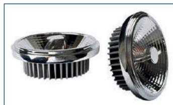
Fittings with 50W halogen lamps can be directly replaced by PEGASUS fitting with 10W LED unit. Reflector of LED unit designed to prevent glare and the LED is hidden behind the metal bracket and the light beam is reflected, softened and focused to a beam angle of 8, 24 or 35 ° degrees.
